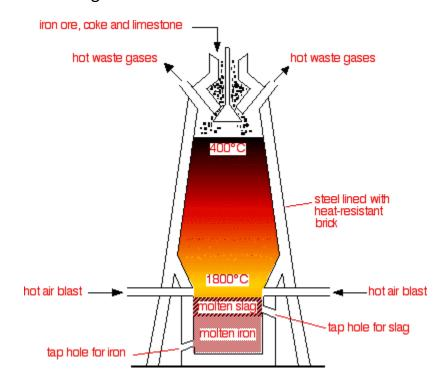
The iron the flows out of the furnace are called **cast iron**. It contains 4% carbon and other impurities like silicon, sulphur and phosphorous.
